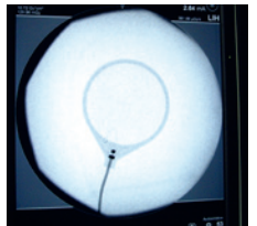
A 60cc ion chamber in the beam.
